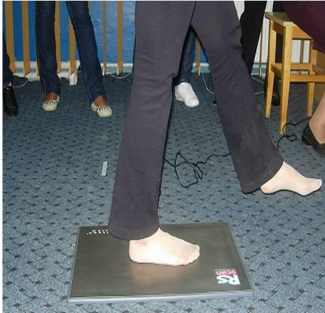
Fig. 9. The use of the Footscan plate: a) outside of walking route, b) included in a walking route of 6 m.
