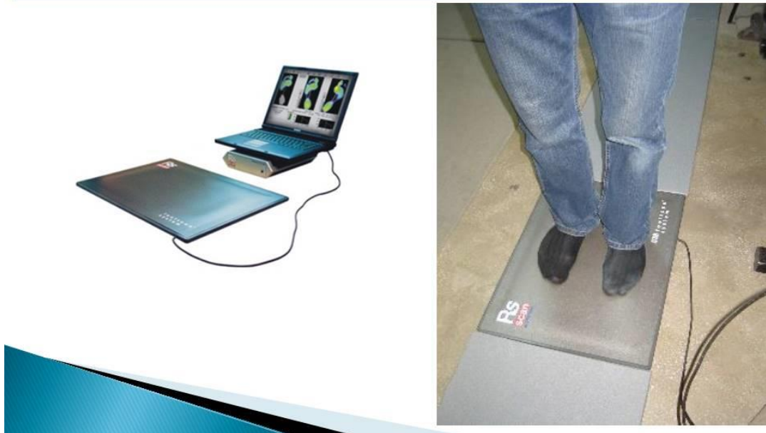
Fig. 1. Footscan system (left). Static measurement with Footscan plate (right).
